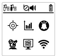
Press both the Up and Down keys simultaneously on the main screen to open the configuration menu on the left. The selected icon will be highlighted with a border. Use the Up or Down keys to navigate to the desired option, then press the Enter key to select it. The settings are available in the following order: Calibration  $\rightarrow$  Measurement  $\rightarrow$  Alarm  $\rightarrow$  Log  $\rightarrow$  Monitor  $\rightarrow$  Wireless Settings.
