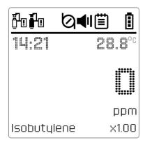
After the device stabilizes and switches to normal measurement mode, the gas concentration and battery power level will be displayed on the LCD screen. The gas concentration is shown in ppm(or ppb), and the value is updated in real-time as the concentration level changes.
